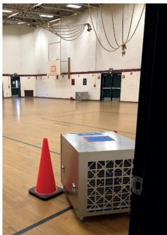
L- large portable HEPA filter unit in Gym. C & R- smaller and quieter EnviroKlenz portable HEPA filter/ UVC light units were found throughout the school.
