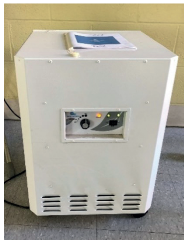
L- large portable HEPA filter unit in Gym. C & R- smaller and quieter EnviroKlenz portable HEPA filter/ UVC light units were found throughout the school.
